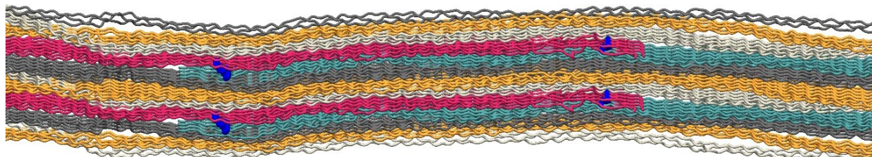
Figure 2: Exemplary atomistic model of a Collagen type I fibril fragment. It comprises 41 triple helices spanning one central overlap and one gap region (in two parts, left and right). Triple helices are colored according to the staggering distance, crosslinks are shown in blue. The regions around these covalent connections turn out to be mechanical weak points in our simulations.
