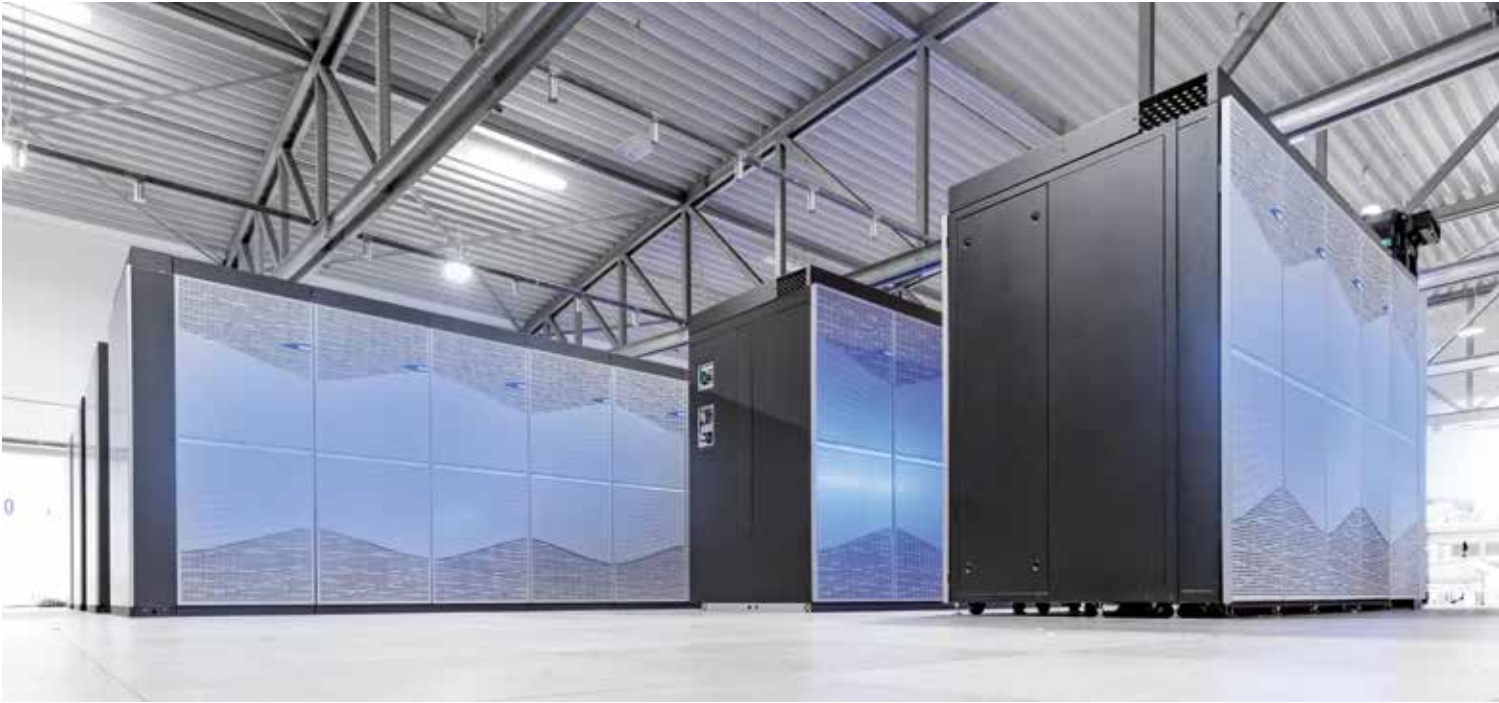
The GPU-accelerated JUWELS Booster module, installed this year, brings the modular machine’s peak performance to roughly 85 petaflops. © Forschungszentrum Jülich
