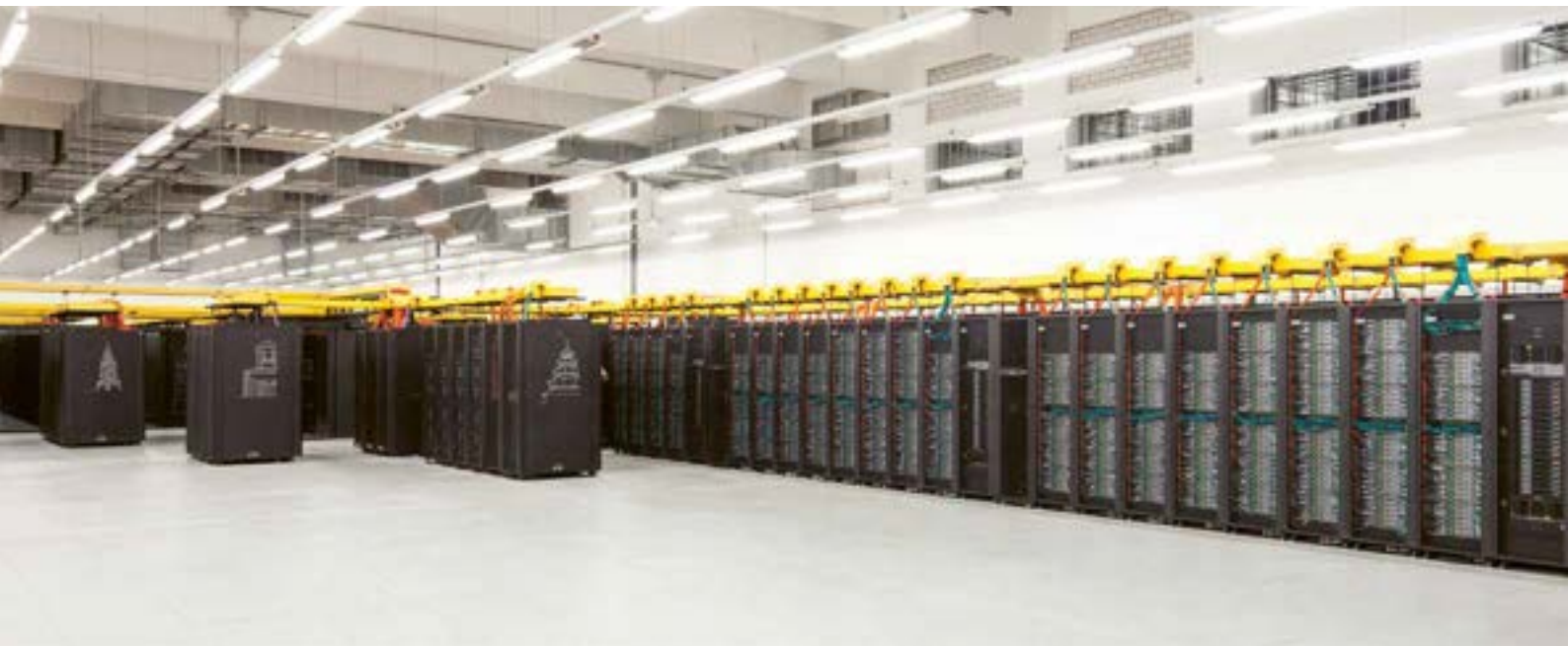
SuperMUC Phase 1 and 2 ran from 2012 to 2018. Phase 1 started out as Europe's fastest system and was the first hot-water cooled supercomputer worldwide when entering the Top500 in 2012.
