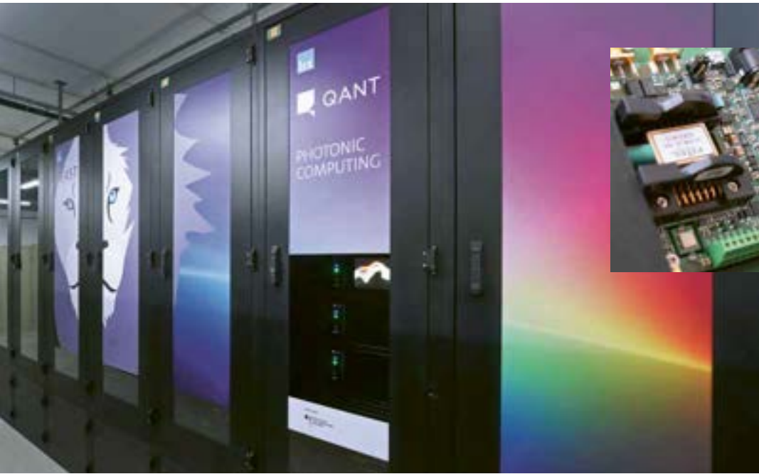
The first installation of a photonic server in a real-live data center environment. The system consists of 3 servers and the technology will be evaluated by LRZ's Future Computing team.
