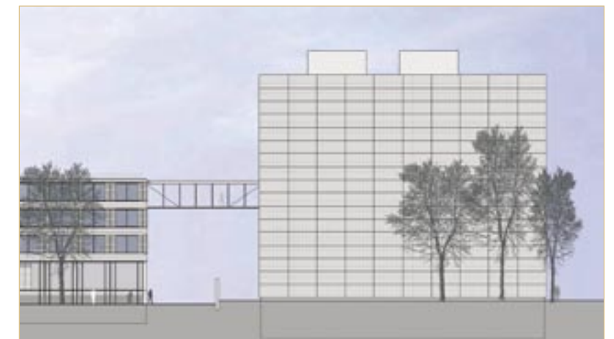
Figure 2: New 36x36x36 meter cube for the computer equipment
