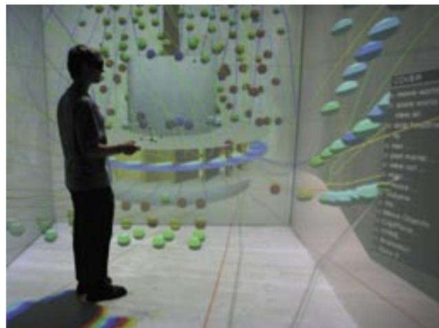
Figure 9: Online simulation of water flow in Kiebingen wicket gate in the CAVE
