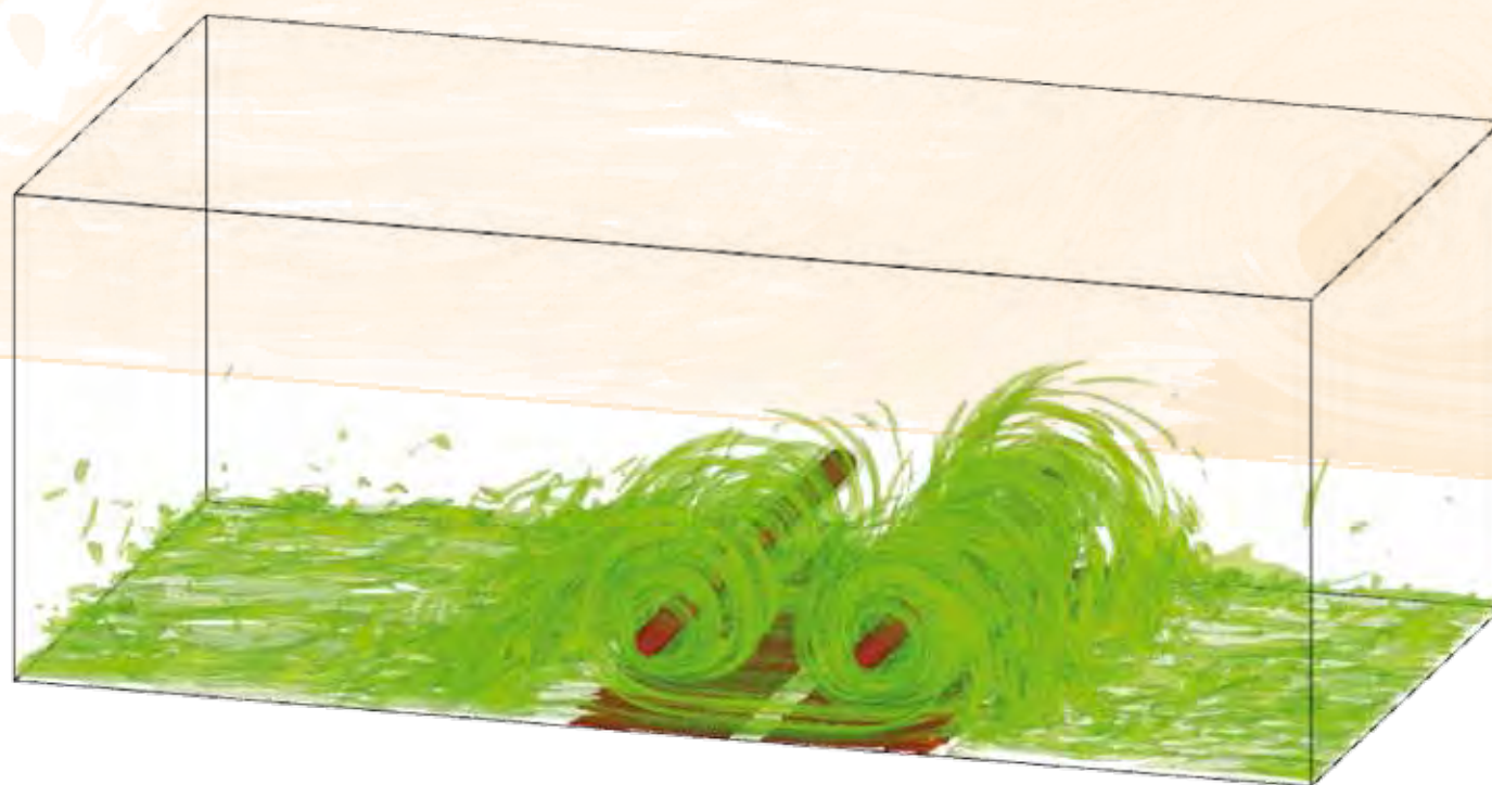
Figure 1: Wake vortex evolution with crosswind in ground proximity. Green vorticity structures representing the crosswind turbulence are being wrapped around the wake vortices (brown vorticity tubes).
