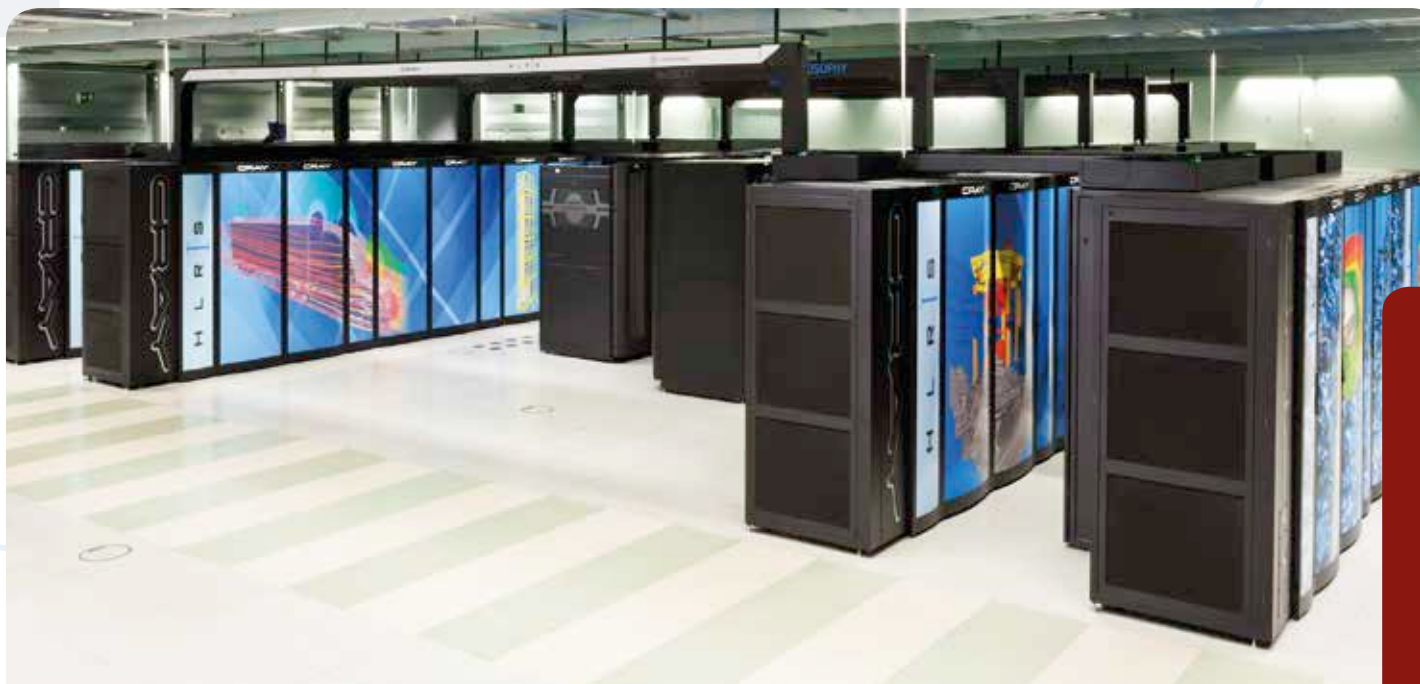
HPC system Hazel Hen of HLRS delivers a Linpack performance of 5.64 Petaflops.
