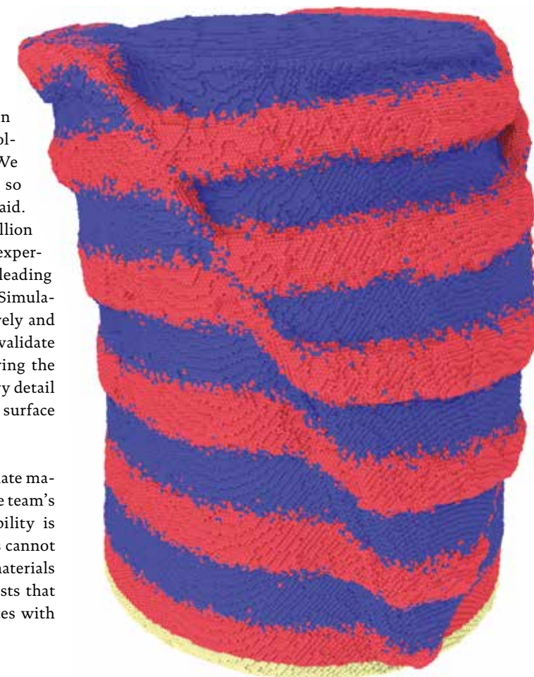
Snapshot of the molecular dynamics simulation of the deformation of a Cu/Au nanolaminate pillar. The image shows the extrusion of a wedge-shaped region. The wedge is bounded by two shear-bands that are the origin of this failure mode. © Adrien Gola
