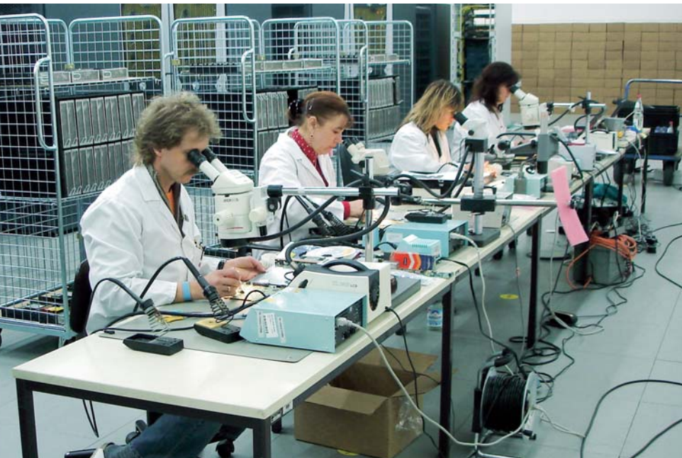
Manual Labor: preparing the SGI Altix 4700 blades for the processor upgrade in the LRZ computer room
