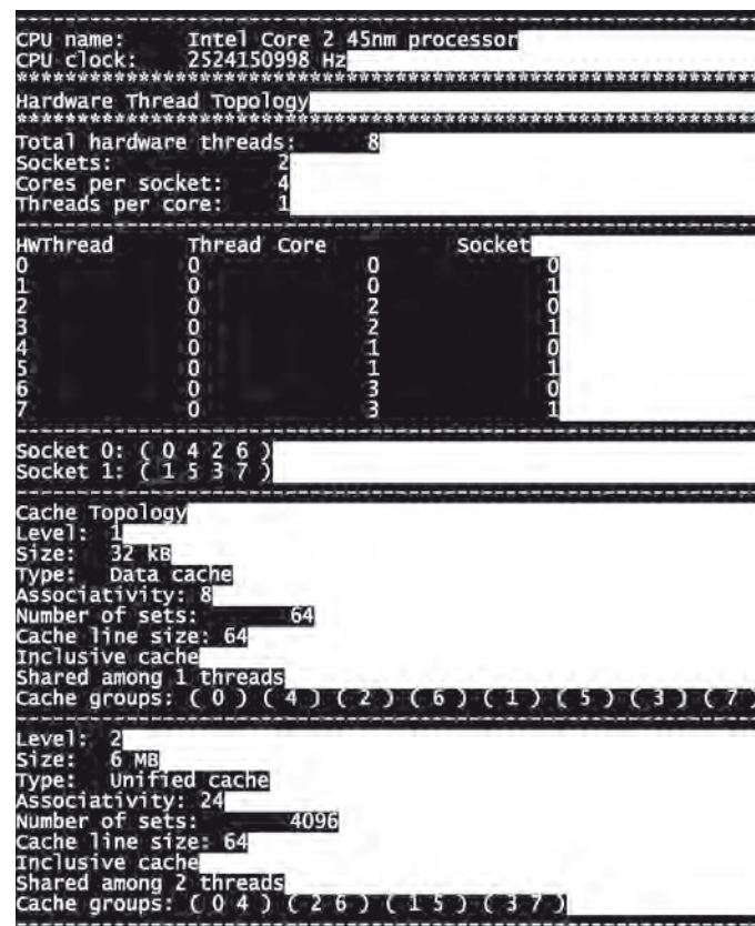
Figure 5: Output of likwid-topology for Intel Xeon node with two sockets
