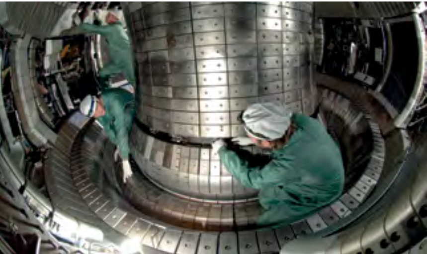
Figure 1: Plasma vessel of the ASDEX-Upgrade tokamak at IPP. © IPP, Photo: Volker Rohde
