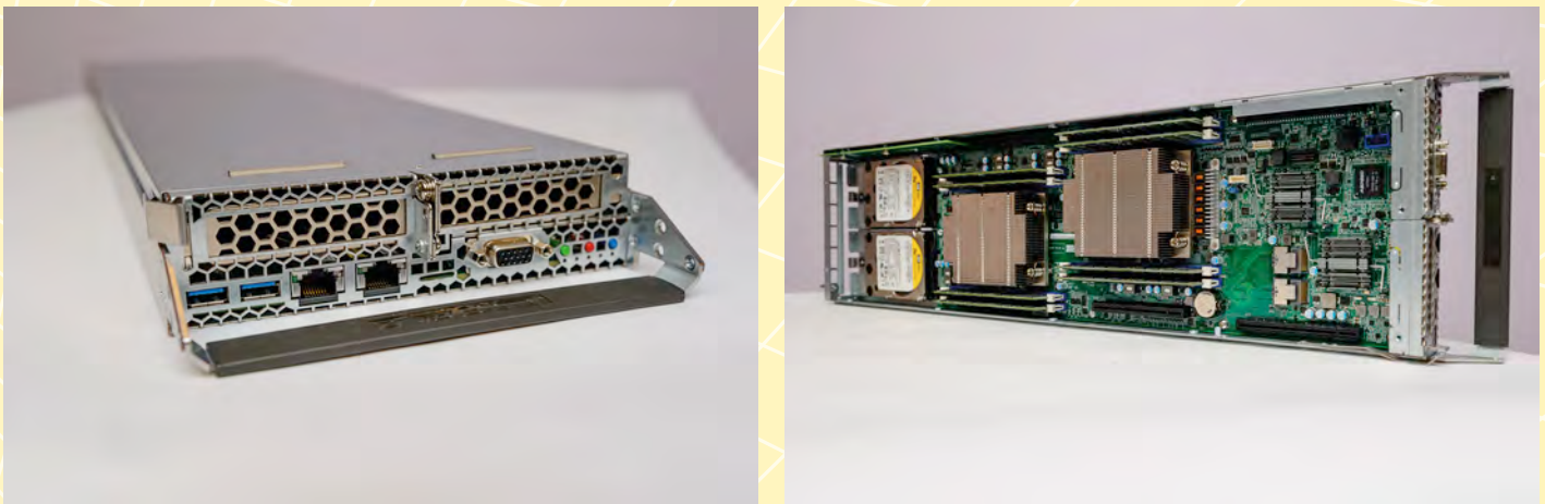
Figure 2: A V210S compute node as used in the JURECA cluster. Each node hosts two CPU sockets. The V201F version, which has twice the width of a V201S module, can additionally host two PCIe-based accelerator cards.
