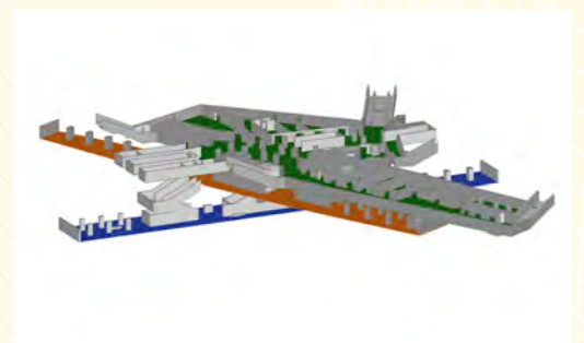
Figure 1: Typical metro stations are complex and compact structures. Hot smoke and passengers have in general the same movement paths to the surface. The figures illustrate the metro station "Osloer Strasse" in Berlin.
