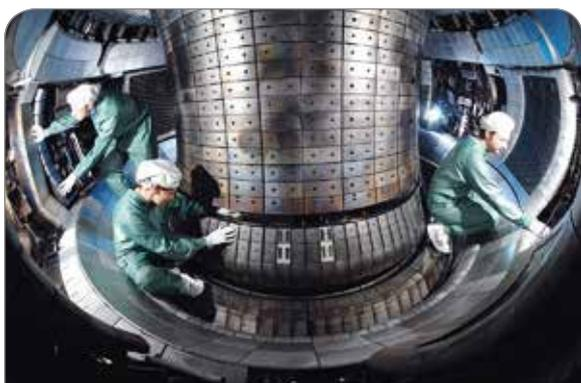
Fig. 1: The interior of the tokamak (torus-shaped) fusion reactor at the Max Planck Institute for Plasma Physics in Garching, Germany. (Image: IPP; Volker Rohde)
