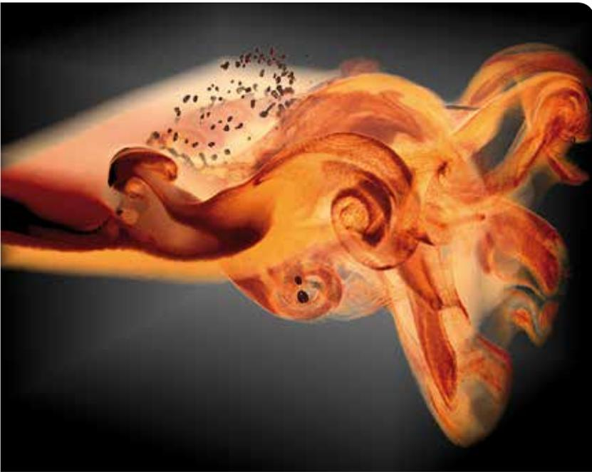
Fig. 3: Development and deflection of the gaseous boundary layer. Volume rendering of the mapped particle IDs, 360 million voxels are used for visualization.
