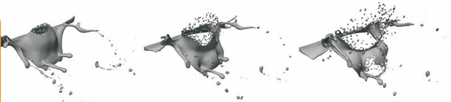
Fig. 1: Sequence of a bag breakup event. The time increment between two consecutive images is 75 microseconds.
